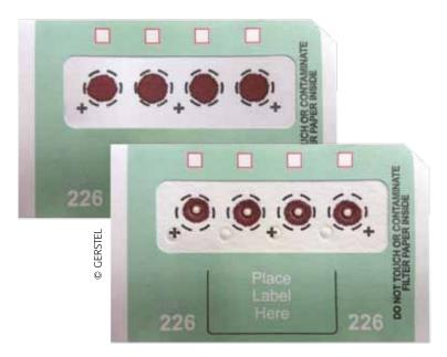
DBS desorption is performed with high accuracy in the user-defined section of the blood spot. Quantitative recovery is achieved resulting in high reproducibility.
